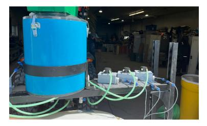
The biocontrol agent in the blue barrel is hooked into the existing spray equipment with the green hoses channeling the agent through the sprayers. Photo: Daniel Cormier
