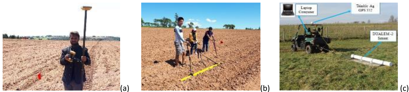
Figure 2: Measurement of ground conductivity using DualEM-II instrument and mapping of selected fields with RTK-GPS.
