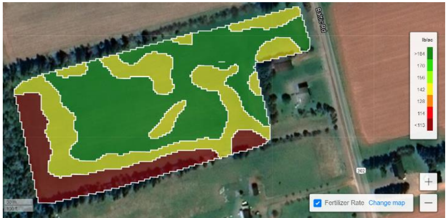
Fig. 2. Management zones for site-specific nutrient management and VR planting in Souris, PEI.
